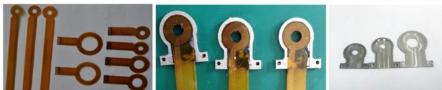
Fig. 4 Grating eddy current micro displacement sensor and smart washer
