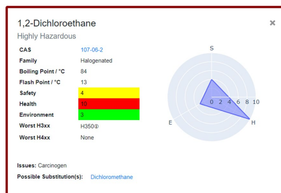
Fig. 3 The solvent flashcard generated for 1,2-dichloroethane. The brown outline corresponds to the CHEM21 ranking: Highly Hazardous
