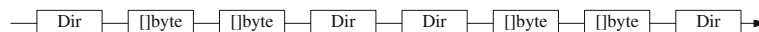
Fig. 2 Example of data streamed through a Clive I/O channel, which can stream a file tree using typed messages. For regular files, file data follows a directory entry. Boxes represent messages
