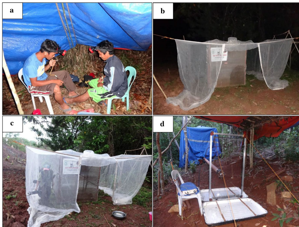
Fig. 2 Mosquito collection techniques used in the study: a human landing catch (HLC), b monkey-baited trap (MBT), c human collectors obtaining mosquitoes from the MBT, d electrocuting net trap (HEN and MEN)
