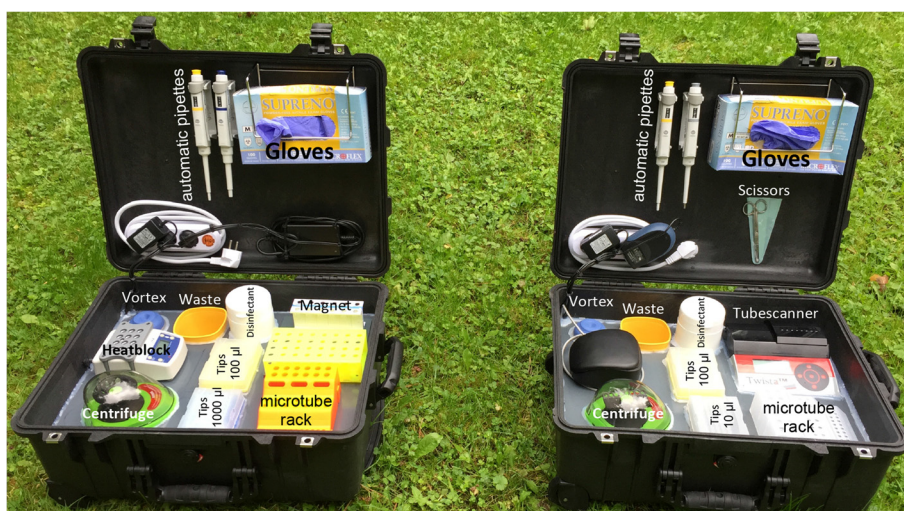
Fig. 1 The mobile suitcase laboratories. The mobile set up was built to host all reagents and equipment to perform the SpeedXtract (left suitcase).
