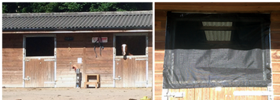
Fig. 4 Field Trial Two: Stable type utilised in field trial two to investigate the effectiveness of insecticide-treated mesh in preventing entry of Culicoides as measured by miniature Ultraviolet (UV) Center for Disease Control (CDC) light-suction traps. One UV light-suction trap was located within each stable whose entrance was either (i) covered with insecticide-treated mesh, (ii) covered with untreated mesh, or (iii) left uncovered without mesh
