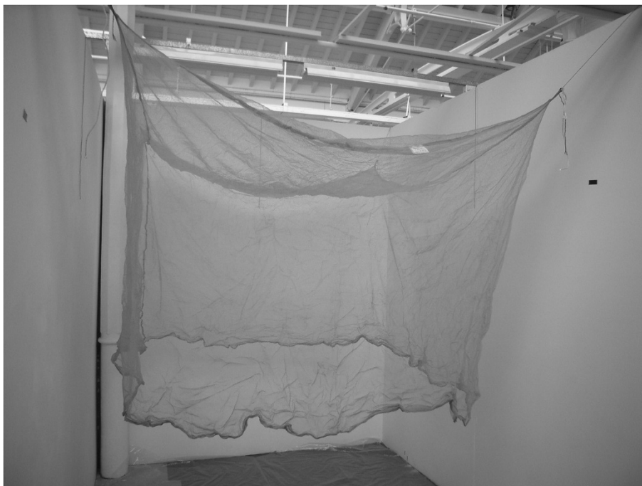
Figure 1 Suspended LLIN for identification of damage.
