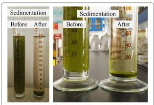
**Fig. 7** Sedimentation of *Graesiella* sp. WBG-1 cells over night. The homogeneous cell suspension (*left*) was kept still in a glass cylinder and over 98 % of biomass sedimented to the bottom after about 8 h (*right*)
