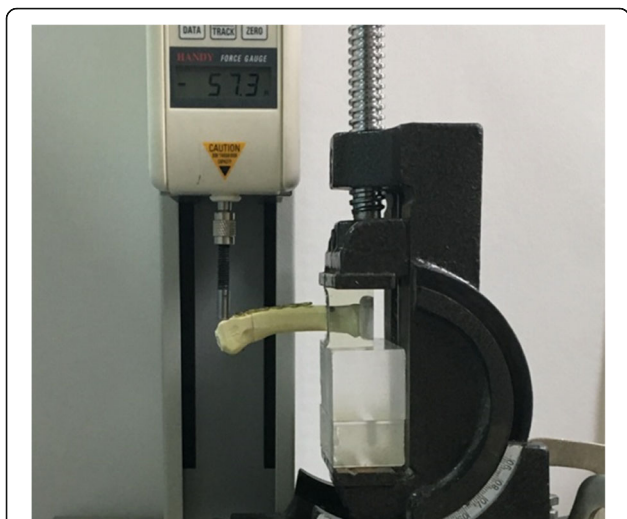
Fig. 3 Experimental setup for cantilever bending tests. The specimen has fixation of a locking plate with five locking bicortical screws
