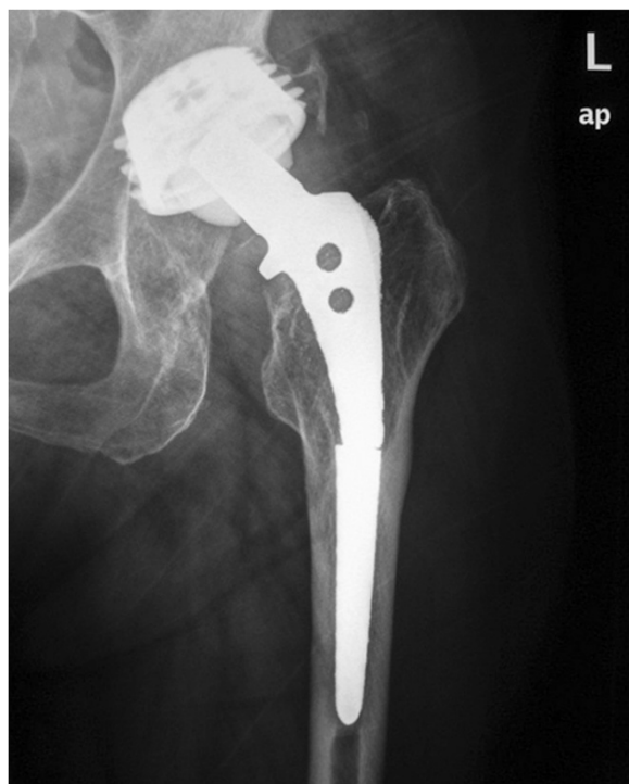
Figure 4 A case of a broken stem with a well-fixed proximal part. A 69-year-old female patient had an Autophor 900S stem implanted 15 years ago. This stem is entirely porous coated and has proximally two fenestrations for better anchoring. The arthroplasty became painful and an anteroposterior radiograph revealed a fatigue fracture of the middle of the stem. The distal part of the prosthesis seems firmly attached to the bone, whereas the stability of the proximal half is uncertain. During operation, this part could not be removed with standard techniques. Taking into account that distally the prosthesis is quadrilateral in cross section, it was decided to be revised with segmentation of the proximal femur.
