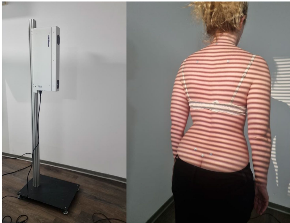
Fig. 1 Three-dimensional back scanner (left) and marker placement (right). Markers are placed on the following landmarks: vertebra prominens (7th cervical vertebra), scapular angle right, scapular angle left, dimple right, dimple left, sacrum point (beginning of the rima ani)
