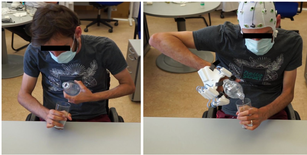
Fig. 5 Participant during baseline (left) and while using a brain/neural hand exoskeleton (B/NHE, right) for the BeBiTT item ‘Pour glass of water’. Without the B/NHE, the participant was unable to securely hold the bottle, so that he had to press the bottle against his torso to stabilize it (left). The B/NHE enabled the participant to firmly grasp and lift the water bottle, allowing him to complete the task without difficulties (right). Control of the B/NHE was established by a hybrid BCI, translating electroencephalographic (EEG) and electrooculographic (EOG) signals into hand opening and closing movements
