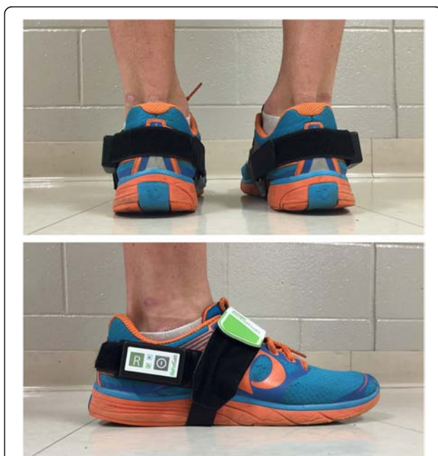
Fig. 1 Photograph showing the sensor placement on the lateral aspect of subjects' personal shoes
