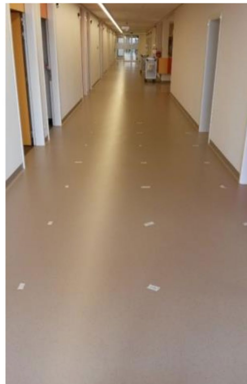
Fig. 6 The mobile node: a Dell laptop with 3 dongles (Wi-Fi, BLE, sensor node STM32) at a trolley at 100 cm height. The ground truth of the evaluation points was indicated on the white sticker on the floor resulting in a grid of 1 m by 1 m. Picture of a room and the corridor
