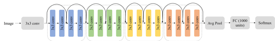
Fig. 7 The ResNet-18 CNN architecture, adapted from [17]
