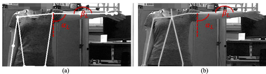
Fig. 3 The (a) Mediapipe and (b) Cubemos frames showing \alpha and \beta angles of S9 at a full SAL
