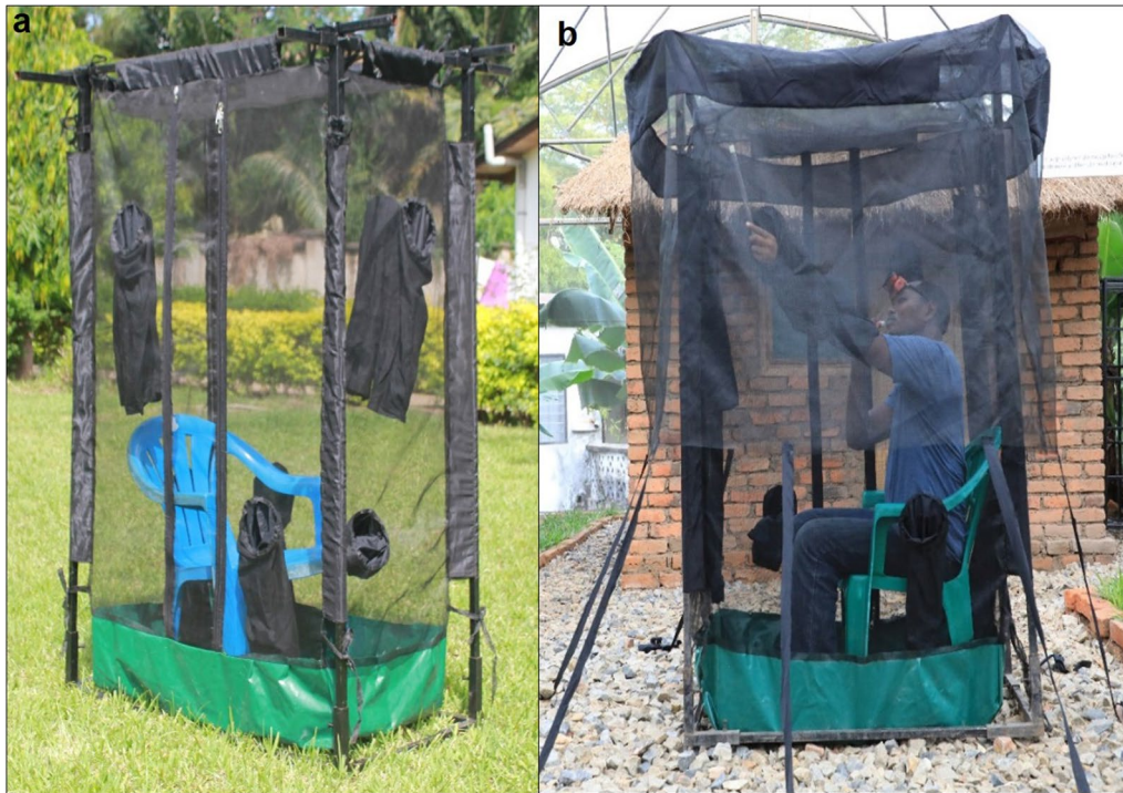
Fig. 3 Pictorial representation of the miniaturized double-net traps (DN-Mini), showing an adult male volunteer occupying the inner compartment
