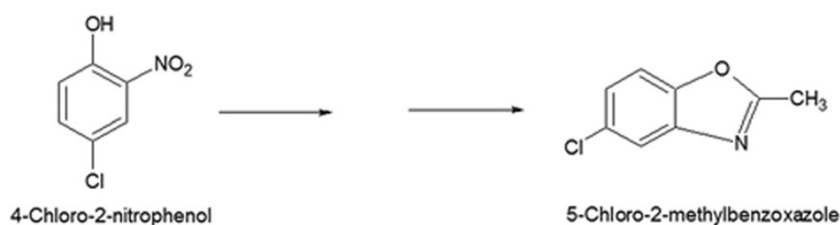
Figure 5 A graphic representation of transformation of 4-chloro-2-nitrophenol into 5-chloro-2-methylbenzoxazole.
