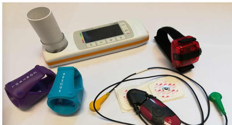
Fig. 2 The smart monitoring devices. Legend: Smart devices from top-left to bottom-right: MIR spirometry II advanced, Actigraph WGT3X-BT, Cohero Health smart inhalers, eMotion Faros 180
