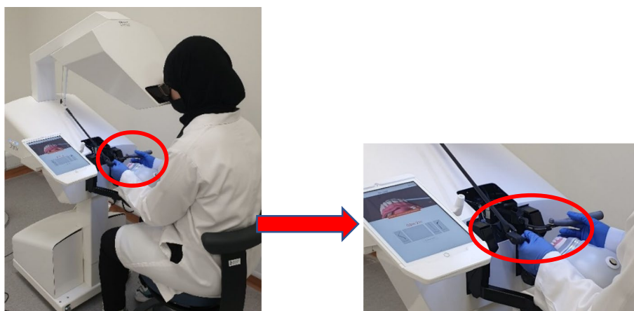
Fig. 1 Virtual reality haptic simulator and handpiece
