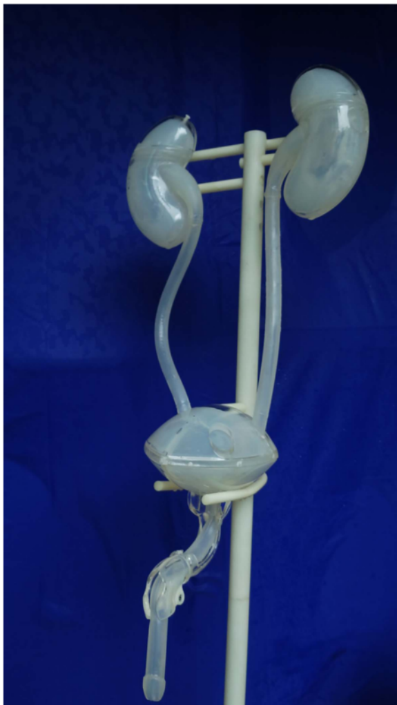
Fig. 2 The assembled transparent simulator, configured to simulate male urinary anatomy
