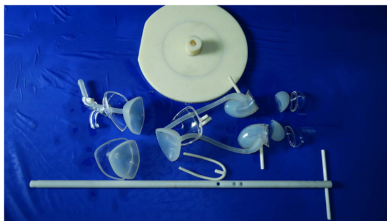
Fig. 3 All components of the transparent simulator: kidneys, ureters, bladder, urinary tracts, brackets and base
