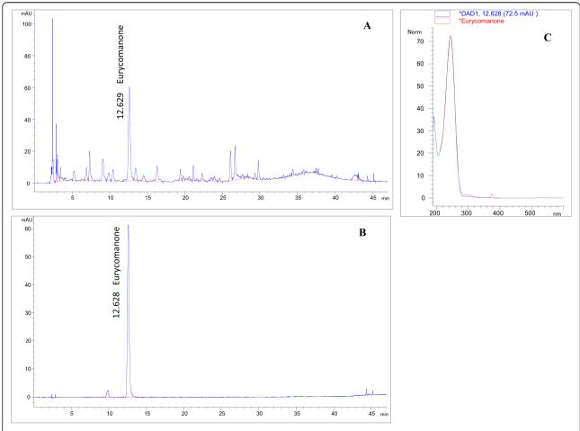
Fig. 1 HPLC profile of PEL water extract. a The major peak corresponds to Eurycomanone at RT 12.629 min. b Eurycomanone standard eluted at RT 12.628 min. c UV spectrum of Eurycomanone with respect to its retention time
