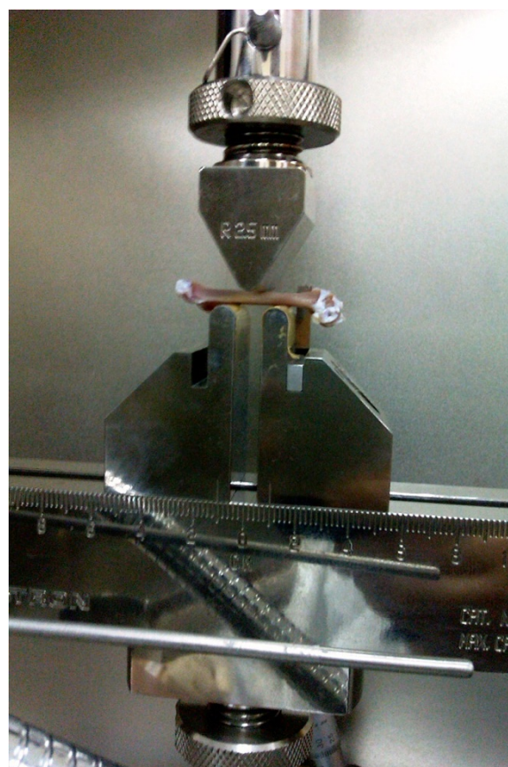
Figure 2 Force applied to the midpoint of the femur.
