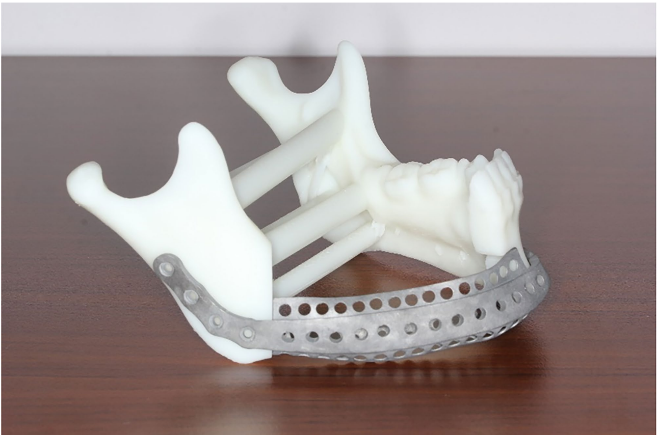
Fig. 3 All models and templates were printed on a 3D printer: osteotomy templates, original mandible model, and titanium mesh
