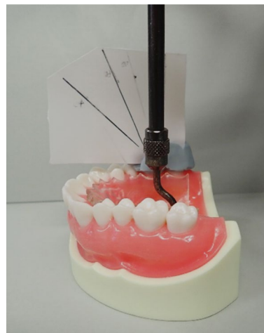
Fig. 4 A device to guide the direction of traction. This device defines 45°, 60° and 90° directions to the occlusal plane
