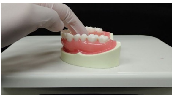
Fig. 3 Pressure welding of the palatal floor to the model on the weighing instrument. The plate was pressure perpendicular to the occlusal plane to the model for 10 s while the load was defined on a weighing instrument
