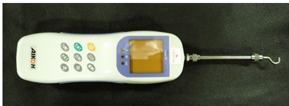
Fig. 2 The measuring device (Digital force gauge RZ-5®;AIKOHENGINEERING, Tokyo, Japan). Measuring the retention of the palatal plate by hooking the tip of the device to a ring and applying traction
