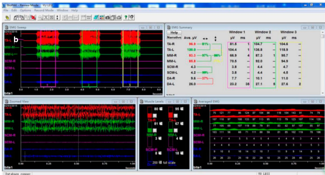
Fig. 1 BioEMG, BioEMG electromyographic amplifier (a) and interface of recording and analysing of EMG (b)
