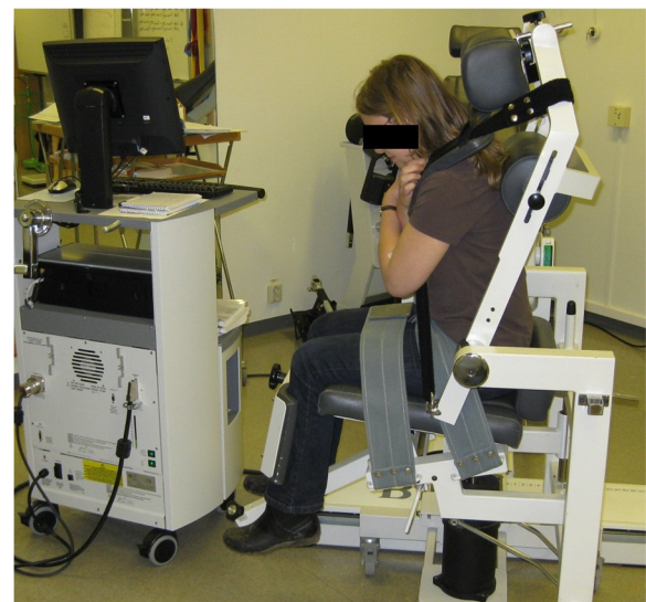
Fig. 1 BioDex, System 4 with the back/abdominal unit. Member of the staff demonstrating Biodex. The patient is strapped in a fixed position. This prevents using other muscles than the abdominal corset and makes it possible to perform tests that are reproducible at a later stage
