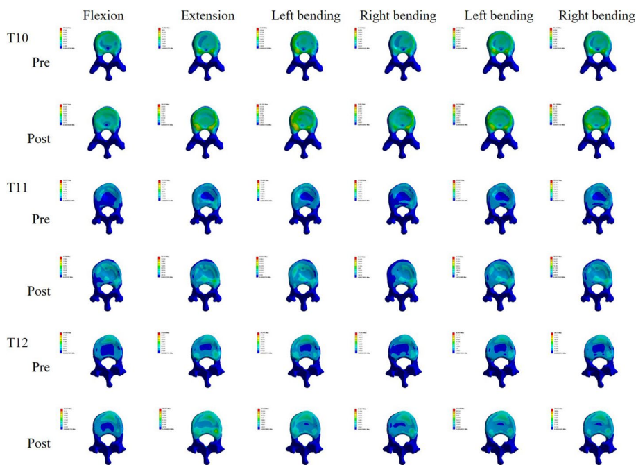
Fig. 3 Stress distribution cloud diagram of wedge vertebral body and adjacent vertebral bodies before and after PPVA. Pre, Preoperative; Post, Postoperative
