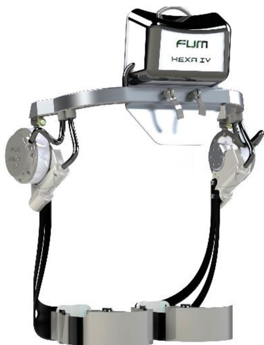
Fig. 1 The powered single hip joint exoskeleton (PSHJE) robots developed in FUM CARE, named HEXA. The robot is portable and weighs less than 4 kg
