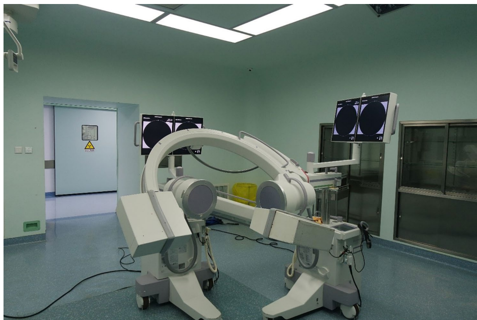
Fig. 2 Dual fluoroscopic imaging system: The DFIS system was composed of two mobile X-ray machines placed perpendicular to each other
