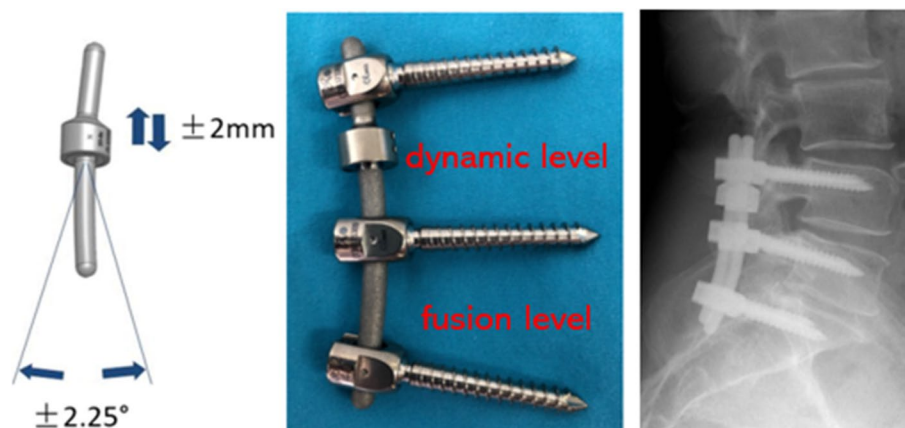
Fig. 1 Hybrid Isobar TTL dynamic stabilization and posterolateral fusion system; the rod has the fixed mobility \pm 2.25^\circ , and the titanium ring with \pm 2 mm longitudinal movement distance
