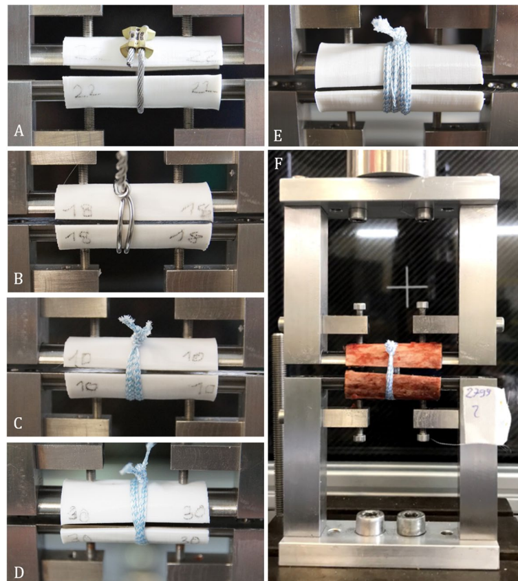
Fig. 1 A-E Displaying all installed cerclage Options on the 3D printed half shell constructs. F Showing the complete biomechanical test set-up with the custom designed grip to individually adjust and place the half shell constructs perfectly into the servohydraulic testing machine
