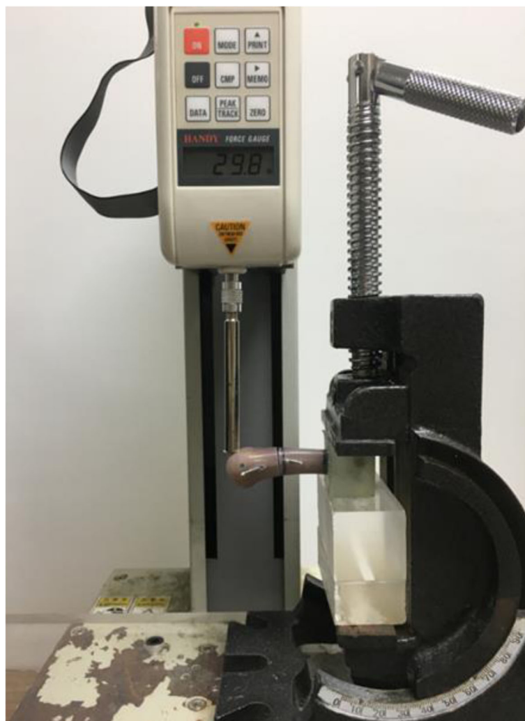
Fig. 4 Experimental setup for the cantilever bending tests
