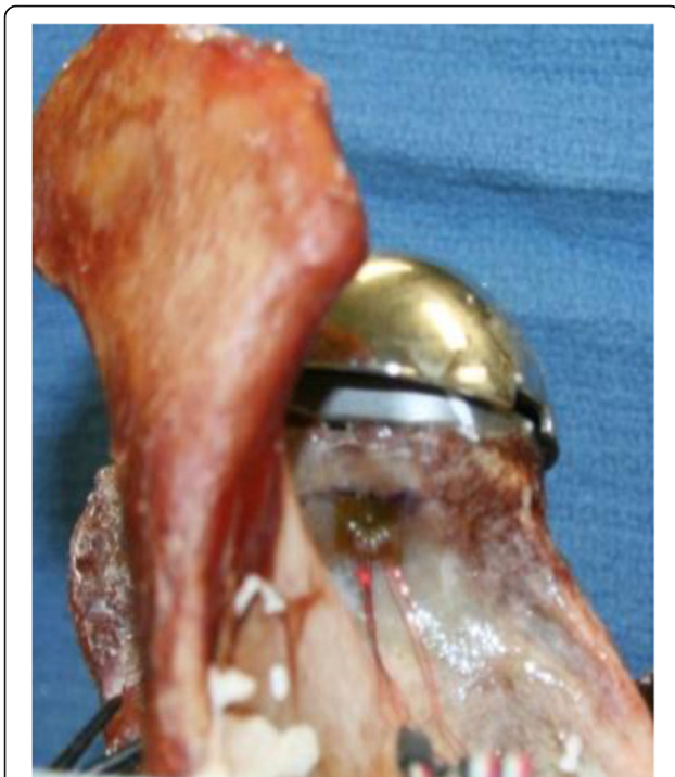
Fig. 1 Superior strain gauge (Vishay, Raleigh, NC) at the 12 o'clock position, 5 mm medial to the reamed glenoid rim
