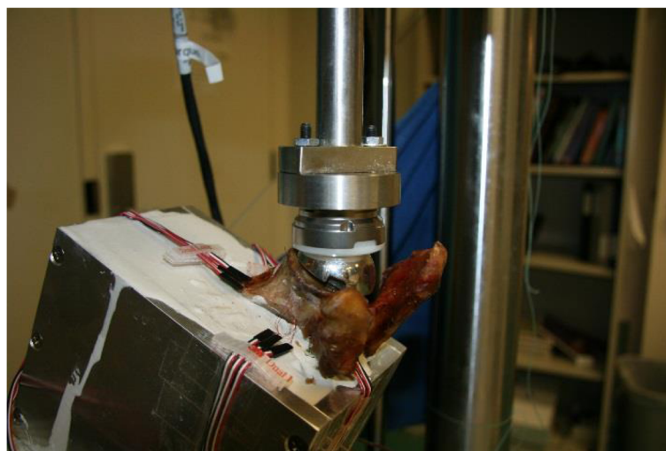
Fig. 3 Biomechanical testing setup showing the mounted scapula with implanted glenoidal components, strain gauges around the glenoid rim, and the humeral component including a polyethylene cup attached via a custom fixation to the actuator
