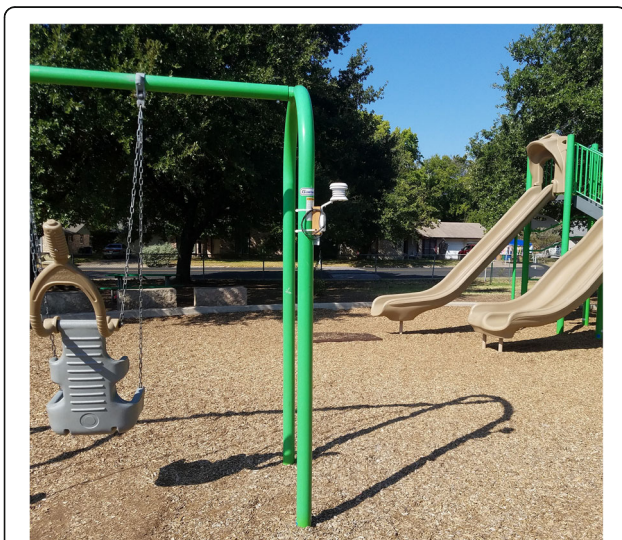
Fig. 2 HOBO MX2302A external air temperature/relative humidity sensor data logger on swing set at low-green park
