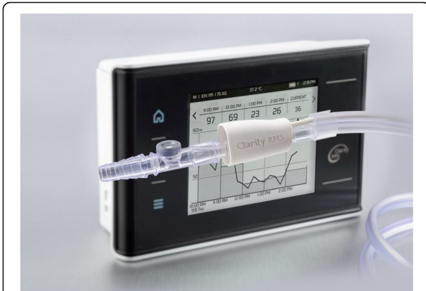
Fig. 1 The RenalSense Clarity RMS Sensor Kit incorporates a proprietary sensor in a standard urinary drainage assembly to monitor urine output as it exits the Foley catheter. The data is communicated to the Clarity RMS Console through a cable integrated within the custom-designed drainage tube to the bag and then to the Console, mounted on the footboard of the patient bed
