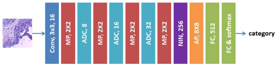
Fig. 3 Network architecture of the proposed atrous DenseNet (ADN). Two modules (atrous dense connection (ADC) and network-in-network (NIN)) are involved in the ADN. The blue, red, orange and green rectangles represent the convolution, max pooling, average pooling and fully connected layers, respectively
