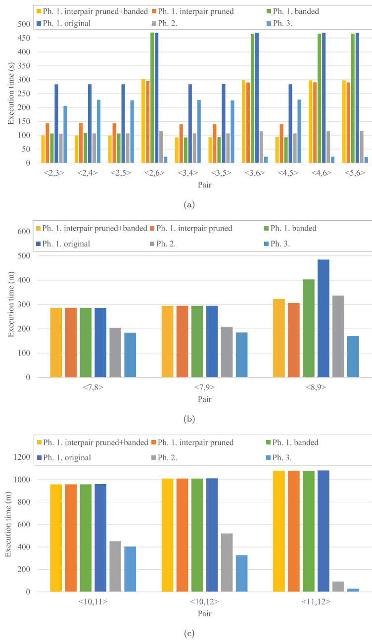
Fig. 12 Breakdown analysis. Breakdown of execution time for genomes of (a) Bacillus anthracis , (b) the human chromosome 21 and (c) the human/gorilla/chimpanzee chromosome 19. The original version of phase 1 corresponds to the score-only Smith-Waterman algorithm with intrapair pruning. Phases 2 and 3 correspond to a banded (score-only) Smith-Waterman algorithm with block pruning and a banded Myers-Miller algorithm, respectively
