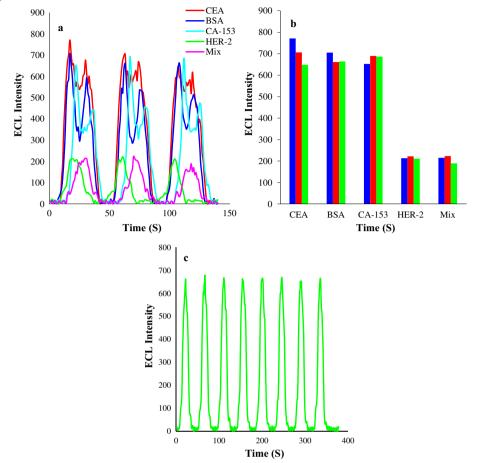
**Fig. 5** a The ECL signals for the possible interferences: BSA, CA-15–3, CEA (0.1 ng mL) in the presence of HER-2 and mixture of them; **b** the related histograms for the selectivity of the proposed protocol for HER-2 quantification; **c** the stability of the designed biosensor in the presence of 1 fM of HER-2 (during 8 repetitive evaluation)
