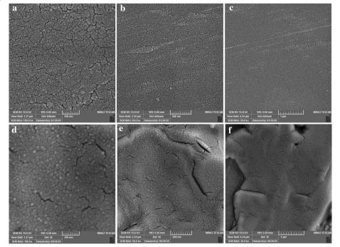
**Fig. 3** The SEM images of the bare electrode ( $\mathbf{a}$ ,  $\mathbf{b}$  and  $\mathbf{c}$ ) and rGO modified electrode ( $\mathbf{d}$ ,  $\mathbf{e}$  and  $\mathbf{f}$ ) at different magnitudes of 200, 500 and 1000 nm
