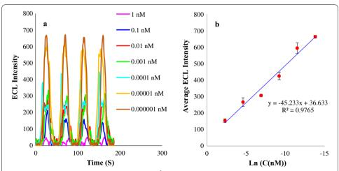
**Fig. 4** a The ECL curves for GCE/rGO/CS-[Ru(bpy) $_3$ ]<sup>2+</sup>/Ab-HER-2 in optimized conditions (pH = 8.2, PBS solution, RT) for different concentrations of HER-2 protein (0.000001, 0.0001, 0.0001, 0.001, 0.01, 0.1 and 1 nM); **b** calibration curve, the ECL intensity of final modified electrode at the corresponding concentrations of HER-2 protein
