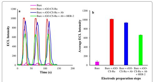
**Fig. 2** Electrode preparation steps. **a** The three consecutive ECL graphs of Bare, Bare + rGO-CS-Ru, Bare + rGO-CS-Ru + Ab and Bare + rGO-CS-Ru + Ab + HER-2; **b** correlated histograms of average ECL intensity
