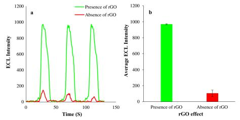
**Fig. 1** The effect of rGO on the intensity of ECL signals. A) The three sequential ECL graphs, in the presence and absence of rGO with the same CS:[Ru(bpy)<sub>3</sub>]<sup>2+</sup> mixture; B) corresponding histograms of average ECL intensity
