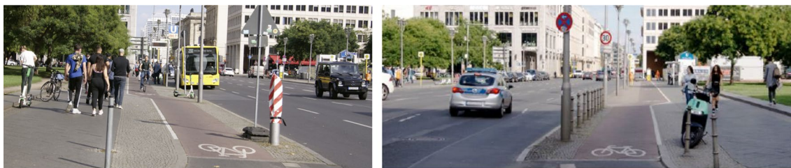
Fig. 4 Site B2 – Berlin, Leipziger Platz; length of observation area: 80 m; off-road bike lane width: 1.5 m (1.9 m at bus stop area); sidewalk width: 3 m; pedestrians per 5 min: 71; cyclists per 5 min: 25
