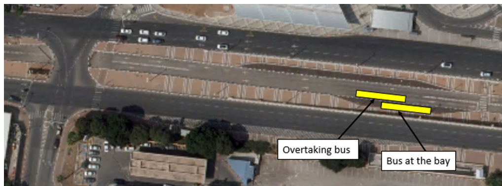
Fig. 2 Example of barrier-separated central BPR with a possibility for bus-overtaking near a bus stop
