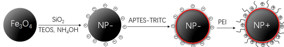
Fig. 1 Design of the nanoparticles. Schematic diagram showing the design of surface-charged, fluorescent, superparamagnetic composite nanoparticles (NPs)
