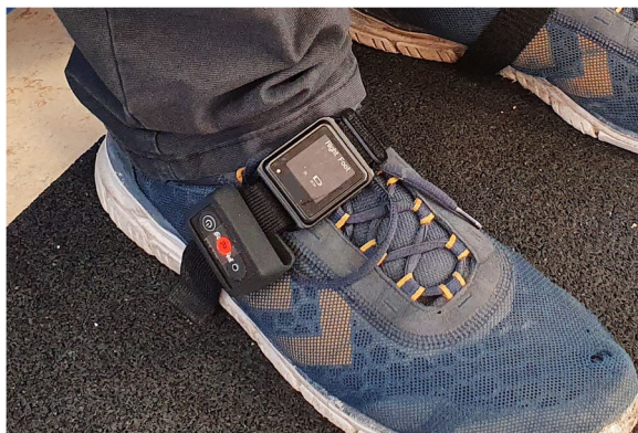
Fig. 1 Image showing the attachment of the inertial sensors of GaitUp and MobilityLab
