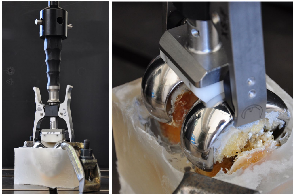
Fig. 5 Visualization of the setup with a specimen mounted for pull-out testing ( left ) and a detailed view of the femoral component clamping ( right )
