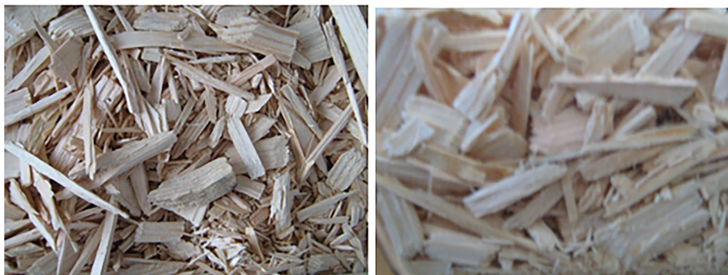
Fig. 1 Wood chips of stem wood used in this investigation, top view (left) and side view (right). The vertical length of each image corresponds to 30 cm. The figure shows dry wood chips. The side view was photographed through a plastic container used in the experiments to get the correct orientation of the wood chips by gravity (hence the blurry image)
