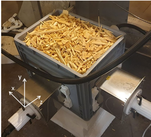
Fig. 2 Sample box—with antenna housings—filled with wood chips. Also shown is the coordinate system used. The antennas (not seen) are rotated inside the metallic boxes to give horizontal or vertical E-field
