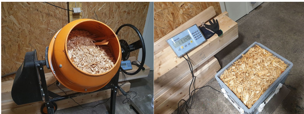
Fig. 3 Cement mixer for moisturizing the wood chips (left) and weighting procedure (right)
