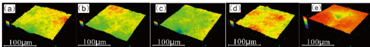
Figure 6 Effect of working pressure on surface topography: (a) 0.2 MPa, (b) 0.3 MPa, (c) 0.4 MPa, (d) 0.5 MPa, (e) 0.6 MPa
