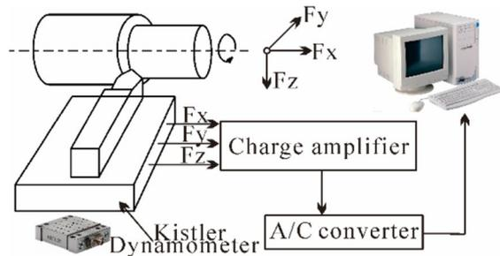
**Figure 4** Schematic illustration of turning experiments
