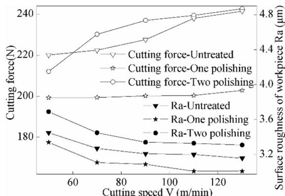
**Figure 12** Effect of cutting speed on cutting force and surface roughness of workpiece
