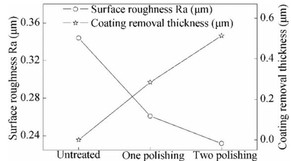
**Figure 2** Results of applying MASJ in multiprocess machining of coated tools
