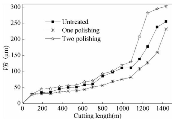
**Figure 11** Wear curves of three types of coated tools
