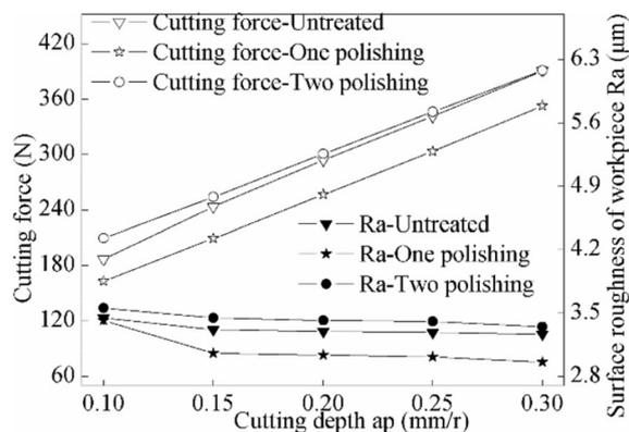
**Figure 14** Effect of cutting depth on cutting force and surface roughness of workpiece
