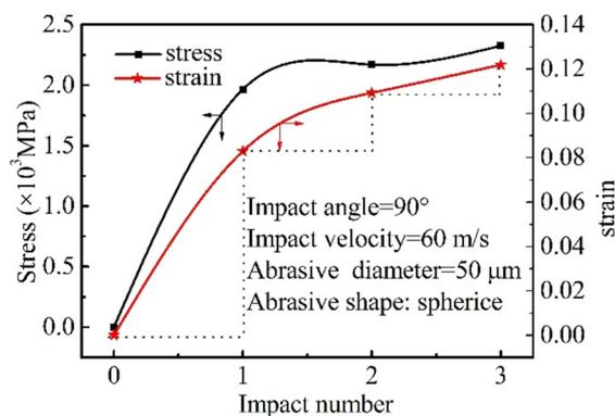
**Figure 10** Effect of multiple impact on stress and strain [26]
