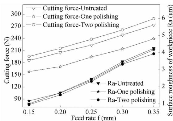
**Figure 13** Effect of feed rate on cutting force and surface roughness of workpiece
