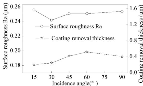
Figure 8 Effect of incidence angle on surface roughness and coating removal thickness
