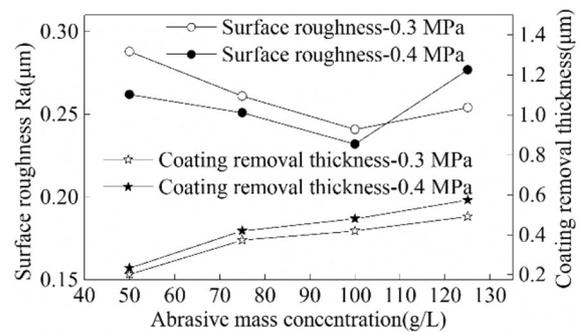
**Figure 9** Effect of abrasive concentration on surface roughness and coating removal thickness
