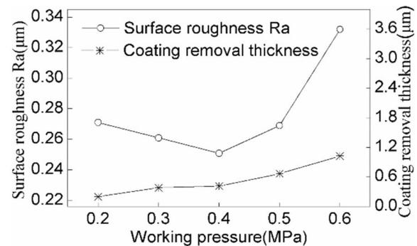
**Figure 5** Effect of working pressure on surface roughness and coating removal thickness
