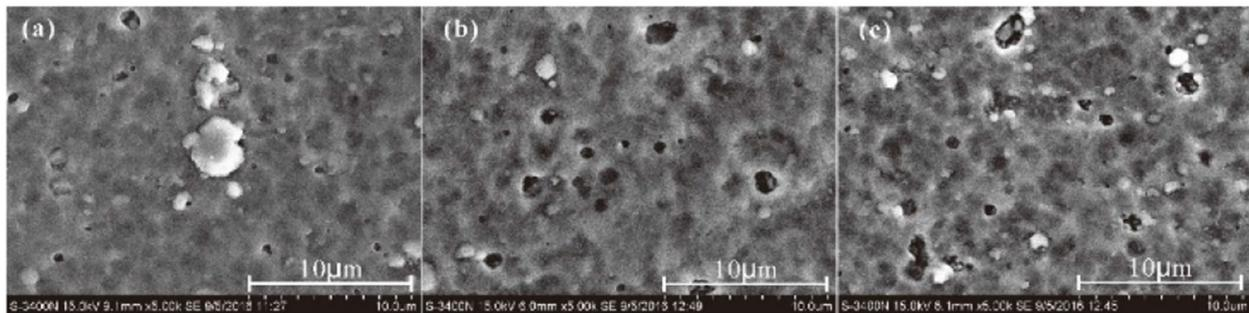
**Figure 3** Surface topography of coating tools after multiple processing: (a) Untreated, (b) One polishing, (c) Two polishing
