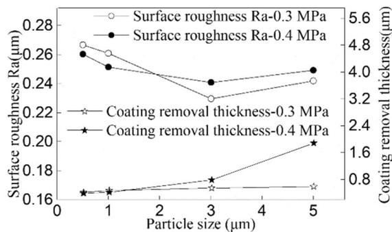
Figure 7 Effect of particle size on surface roughness and coating removal thickness
