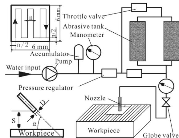
**Figure 1** Principle of MASJ process
