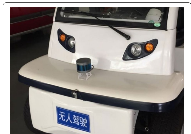
Figure 2 RS-LiDAR-16 installed on our autonomous vehicle
