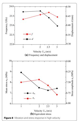
frequency in the velocity range of 1–3 m/s. It means that the vibration frequency exhibits independence on the inlet velocity. As a result, the vibration amplitude is more susceptible to the fluid velocity compared to the vibration frequency.
