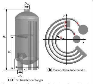
**Figure 1** Heat transfer exchanger with single-row planar elastic tube bundle
