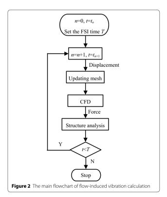
elastic tube bundle is calculated based on the above force boundary. Consequently, the flow-induced vibration of planar elastic tube bundle in shell-side is calculated by this sequential solution of bi-direction fluid–structure coupling method.
