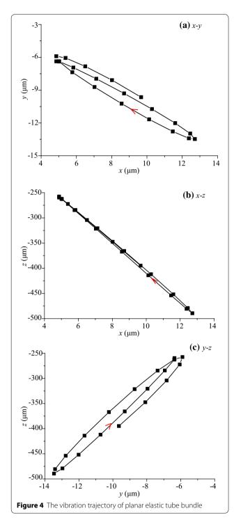
the planar elastic tube bundle is still below the horizontal plane at the position of peak. While the planar elastic tube bundle is almost over the horizontal plane at the position of peak in the velocity 0.5 m/s. The reason behind this is that the fluid force generated by increasing velocity overcomes the effect of earth gravity. It means
