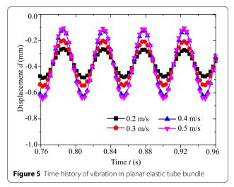
that the vibration balance position will be raised because of the increasing fluid force.
