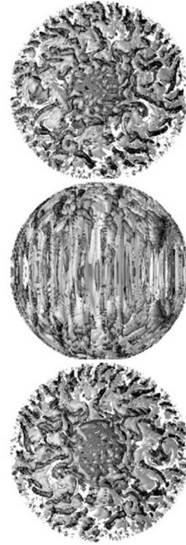
Fig. 7. 3-D views of the convection structure. Drawn are isosurfaces of the axial component of the vorticity ( |\omega_z| = 6000 ) viewed from the north (top), equator (middle) and south (bottom). Positive (negative) value is represented in black (gray).
