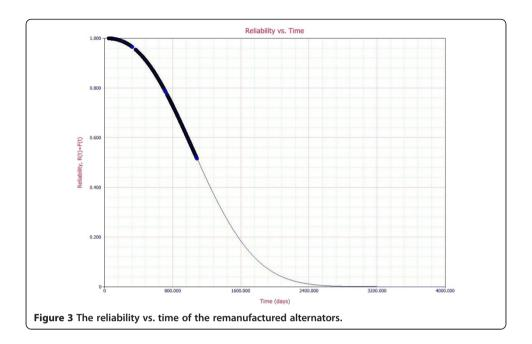
However, the reliability of new product is 100% in the early part of its life and gradually declines during its lifetime [8]. The mean time to failure of the alternator was 1,142 days, and the reliability model of the remanufactured alternator is presented in the following equation:
