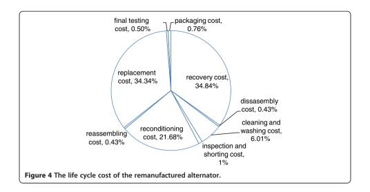
(34.34%), reconditioning cost (21.68%), cleaning and washing cost (6.01%), inspection and shorting cost (1%), packaging cost (0.76%), final testing cost (0.50%), reassembling cost (0.43%) and disassembling cost (0.43%).
